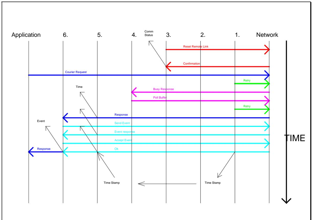
A logical connection is made to the slave device by layer 3 issuing a Reset Remote Link command. Layer 3 identifies that the slave device is present at that address and makes this communication status information available to the application.
