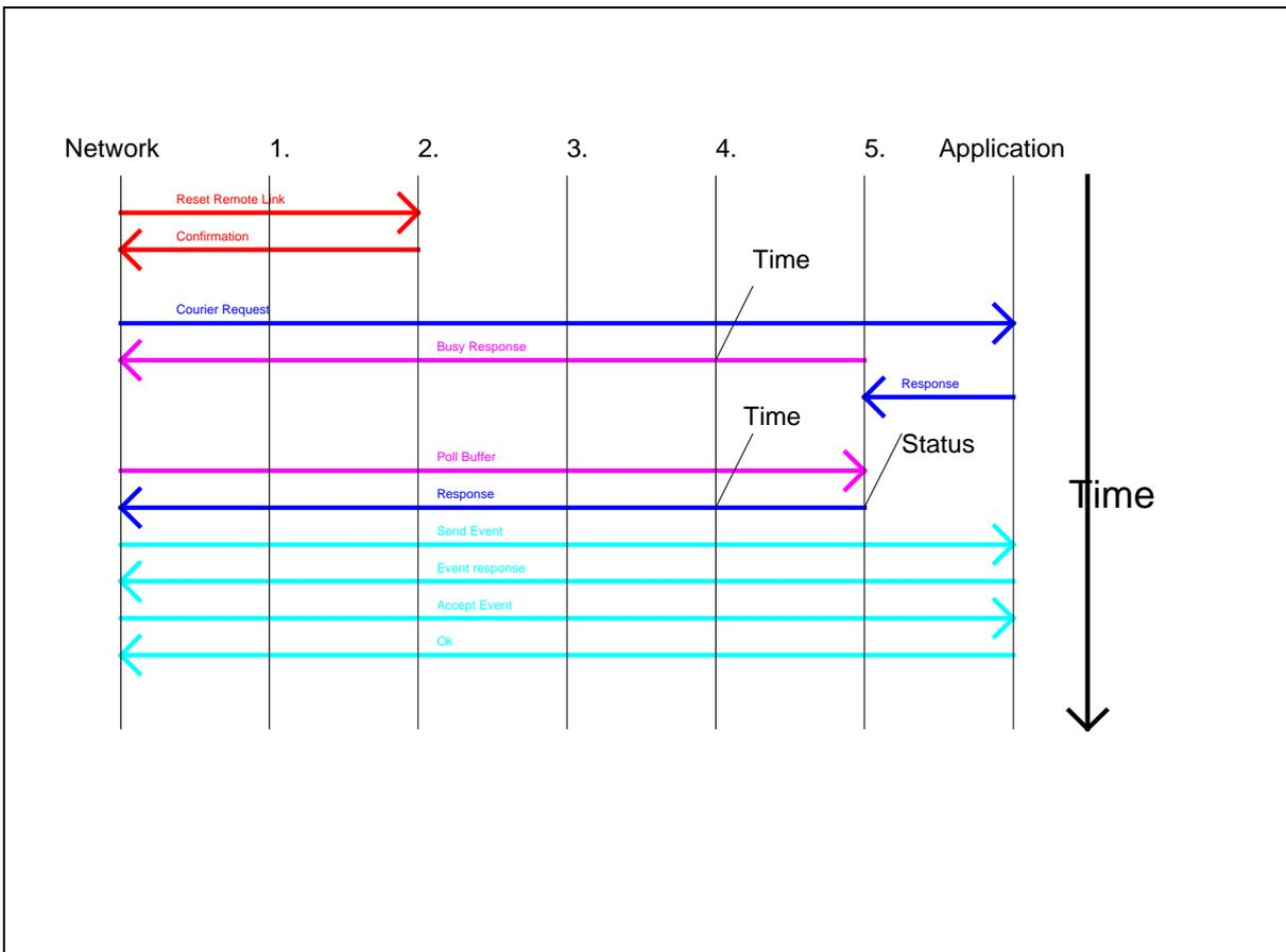
A reset remote link command is received which Layer 2 intercepts and returns a confirmation.
